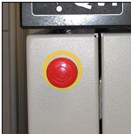
Figure 5-2 E-Stop on the Front of the Machine
