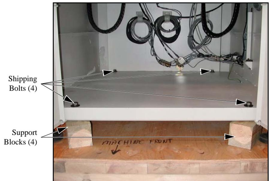
Figure 4-2 Removing the Shipping Bolts that Secure the Machine to the Pallet
