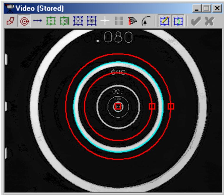
12. Click on the green **Check Mark** in the *Video* window toolbar. VMS calculates X pixel size and inserts this value in the *Define Lens Calibration* dialog box.
