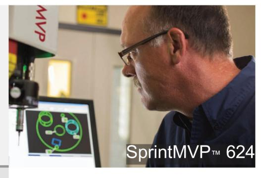
SprintMVP 624 is a fully automatic, 3-axis dimensional measuring machine designed to handle large, heavy parts and fixtures. SprintMVP 624's moving bridge design allows all measurement sensors to be moved out of the way for part loading/unloading.
