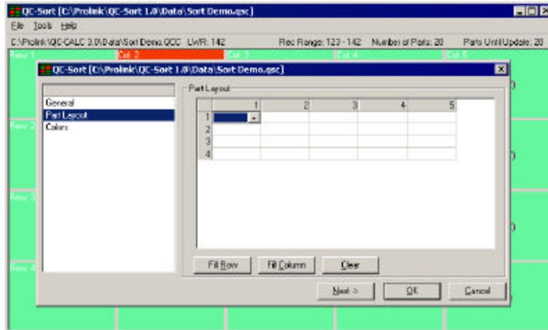
Now manually fill in the numbers in the direction of inspection. Start with part #1 and fill the grid with numbers that represent the order the CMM will travel from part 1 to 20 (in this case). QC-SORT maintains a list of valid numbers and will not let you enter the same number twice.
