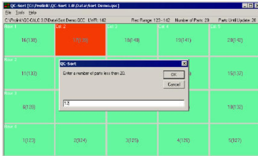
As inspection continues, the screen update occurs but only the partial positions on the fixture are updated after the 12 parts are received. The extra 8 positions are grayed out indicating a partially filled fixture.
