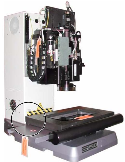
Figure 4-3 Removing the X-Axis Shipping Restraint
