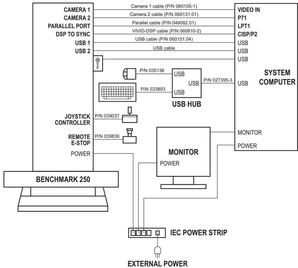
Figure 4-7 System Cabling Diagram (Dual Magnification Systems)
