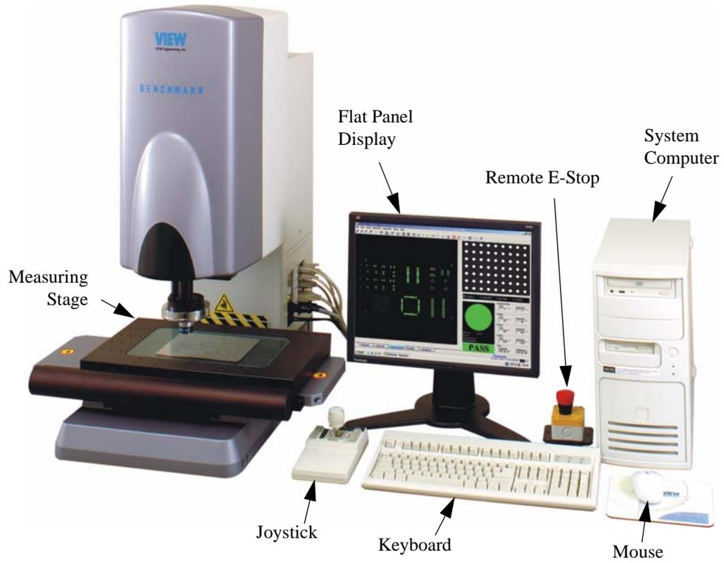
Figure 2-1 Benchmark 250 System Components
