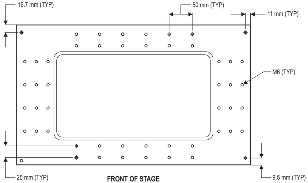
Figure 5-3 Benchmark 250 Stage Fixturing Holes
