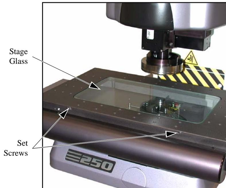
Figure 4-6 Installing the Stage Glass
