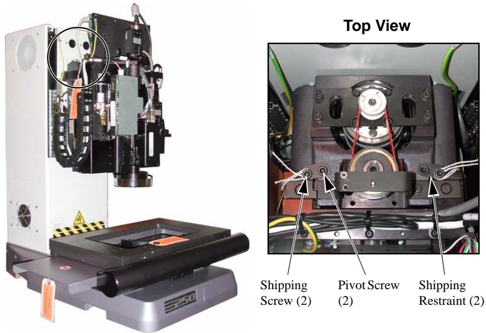
Figure 4-5 Removing the Z-Axis Shipping Restraints
