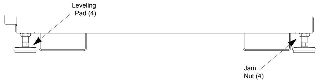
Figure 4-4 Leveling the System
