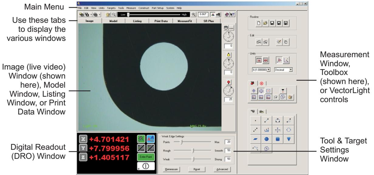
Figure 3-1. Screen Layout - Standard User Interface
