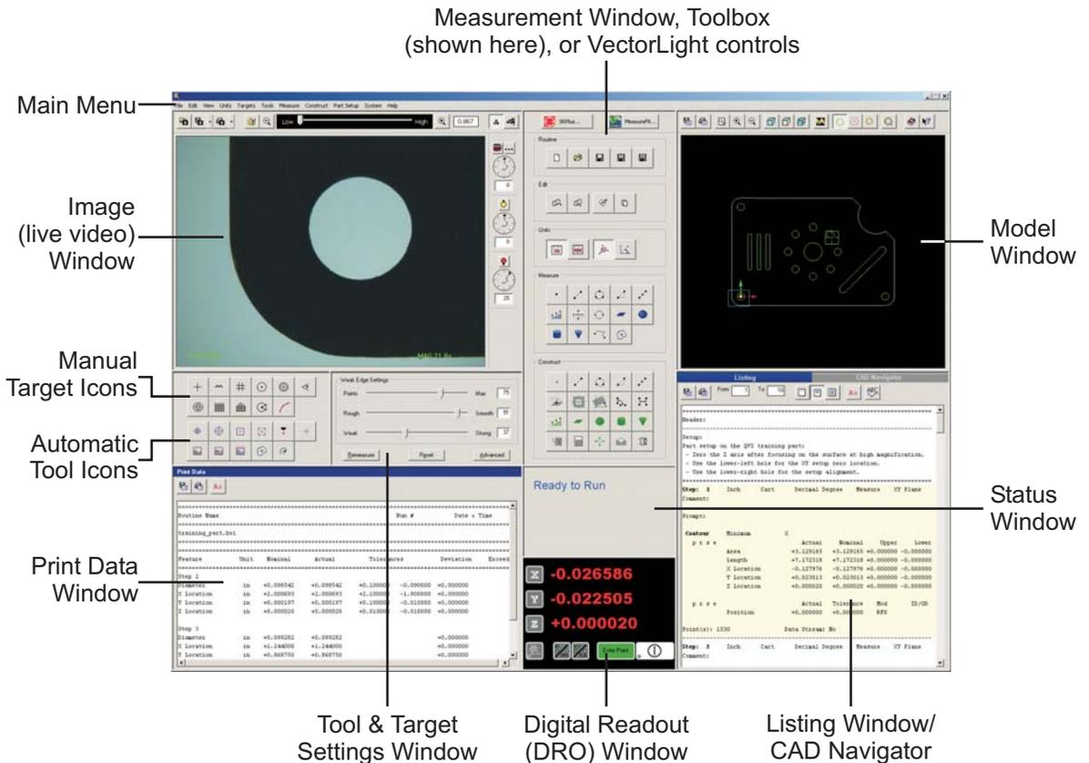
Figure 3-2. Screen Layout - Single Monitor User Interface
